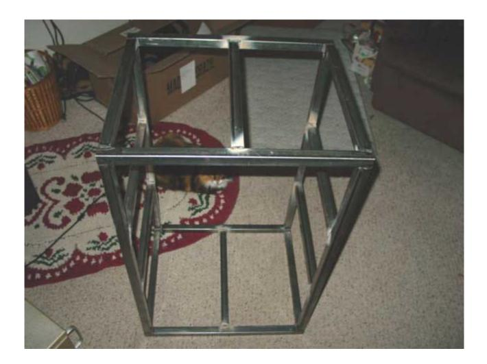
The next step is to weld in the remaining 16" pieces that will serve as supports to reinforce the frame. One per side is centered into the top and bottom, and two into each side. These help distribute weight from the rack rails and help prevent the tubing buckling under extreme loads.
