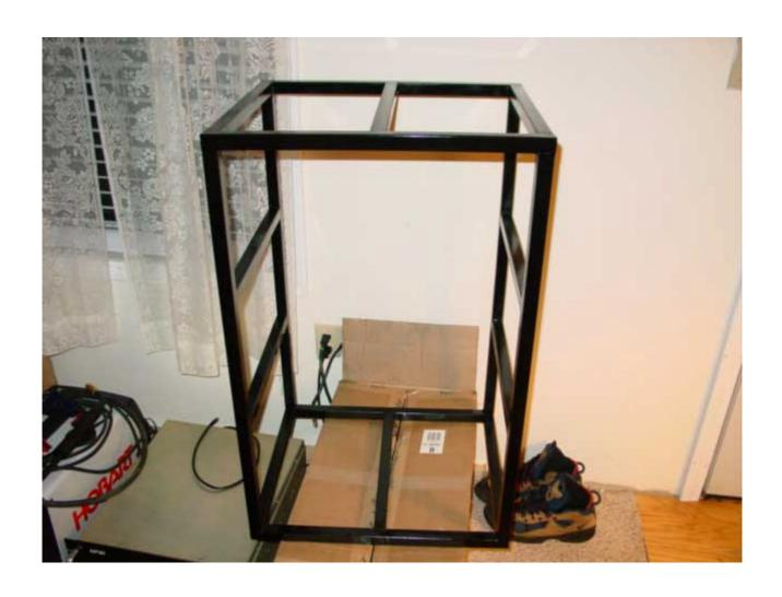
The next steps are to clean the frame thoroughly, and then to paint the frame completely with primer and then a good quality paint. This isn't intended to be cosmetic so much as to prevent corrosion - exposed steel will eventually rust.
