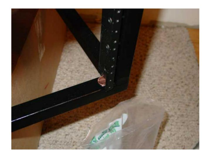
With the frame finished, the rack rails can be mounted. Since the design leaves the rack slightly larger than required, the rails can be centered into the frame vertically by using something to gap the bottom of each rail up from the bottom tubing. A cheap but workable tool for this is an ordinary coin of roughly 1/16" thickness, such as a penny. Simply place a penny on the bottom tubing and stand the rail vertically onto it.
