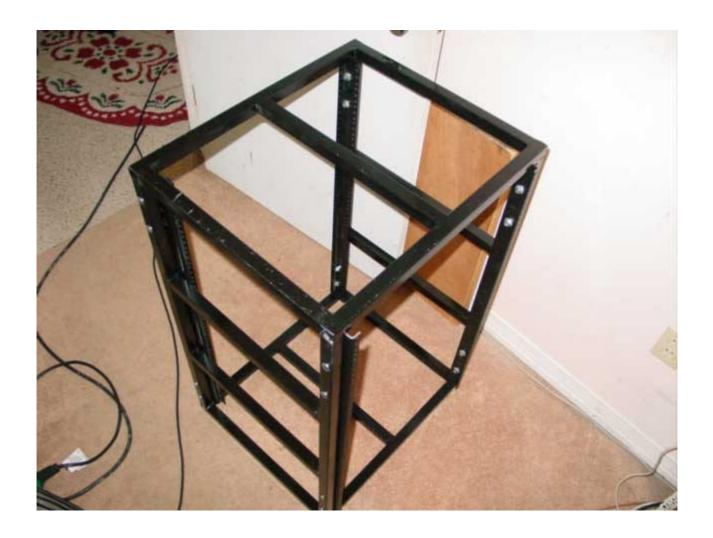
At this point, the rack cabinet frame is complete enough to use as-is, or you can attach side panels to the frame using whatever hardware you need. One nice-looking (if a bit pricey) suggestion is to drill and tap holes and use cap screws to attach the side panels, and use tinted acrylic for the side panels themselves.
