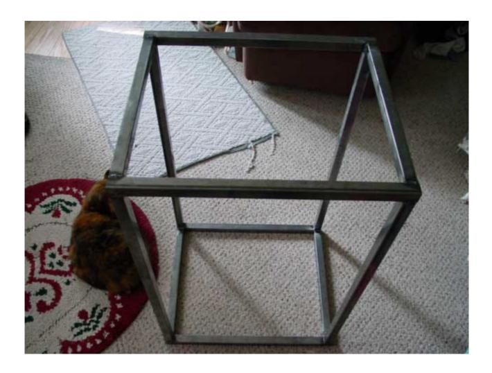
Next, risers are welded at the corners of one of the sections. Again, welding magnets make this easier. When that's finished, the other section is placed onto the risers, indexed properly into place with magnets, and welded to form a basic enclosure.
